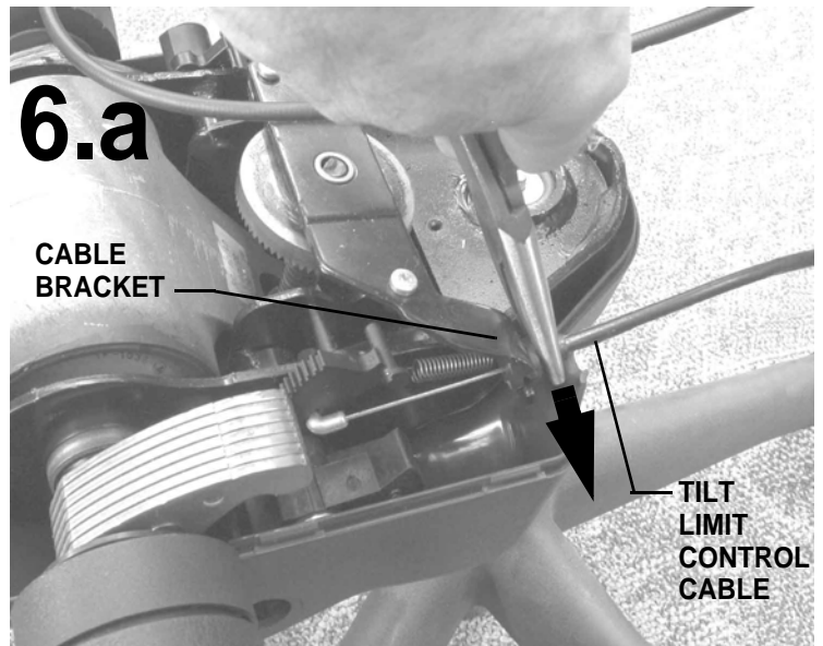
6.a.1 Remove tilt limit control cable by first removing cable from cable bracket with needle nose pliers.
